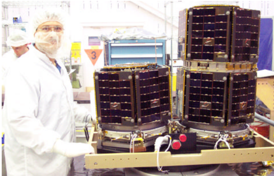
Figure 1 – Completed 3CS nanosats in launch configuration.
