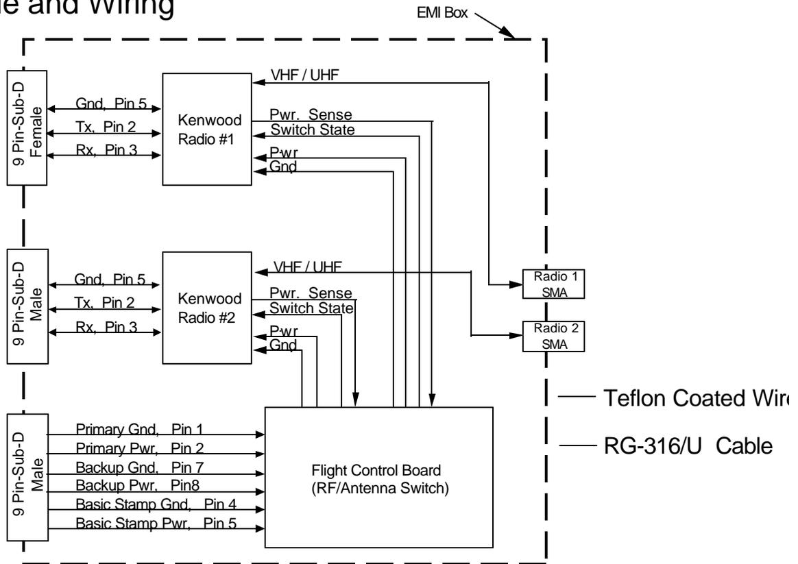
**Figure 4** – Wiring diagram for the flight radio subsystem.
