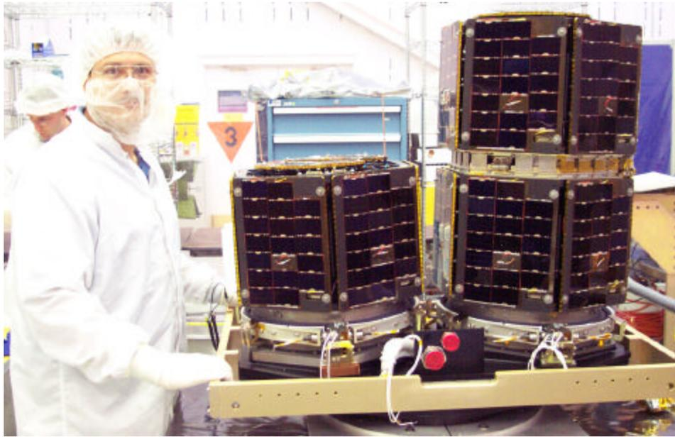
**Figure 1** – Completed 3CS nanosats in launch configuration.
