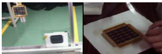
Figure 19 Si Solar Array Panel
