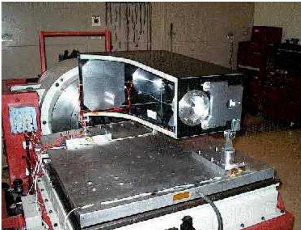
Fig 3 Engineering model undergoing vibration testing
