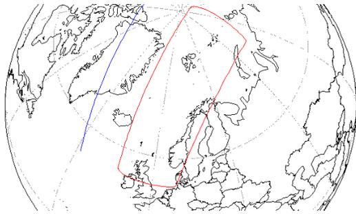
**Figure 4.** 10 min. coverage (red rectangle) obtained from a 600 km polar orbit when the radar detector antenna is pointed sideways. The blue line to the left of the rectangle marks the satellite's ground track.
