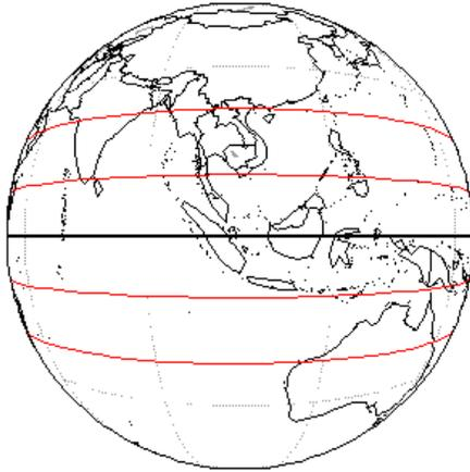
**Figure 11.** The ocean areas between the red lines could be covered 15 times per day from a sideways looking detector in an equatorial orbit. Pointing the detector more along the velocity direction would narrow the coverage areas and move them closer to the Equator.
