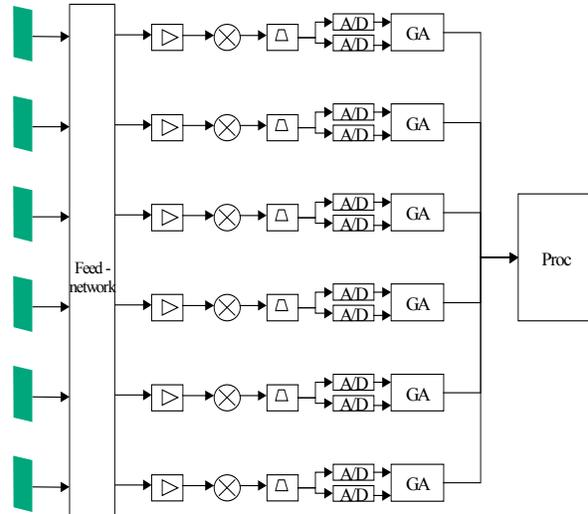
**Figure 5.** Block diagram of the radio interferometer.
