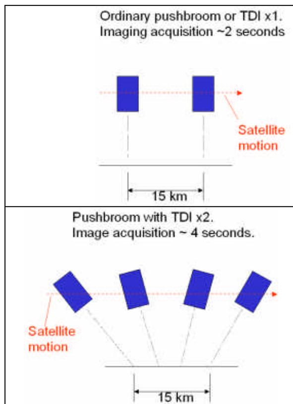
TopSat will be capable of x8 TDI, thus the camera will be oriented to face the target for 8 times longer than an ordinary pushbroom mode. Typically, it will operate using x2 to x4 TDI. In order to achieve this the spacecraft pitch rate will be controlled to within 0.0025°/s (1  $\sigma$ ).
