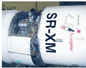
Fig. 4. The TRW Nanothruster Experiment flown on the SR-XM.
