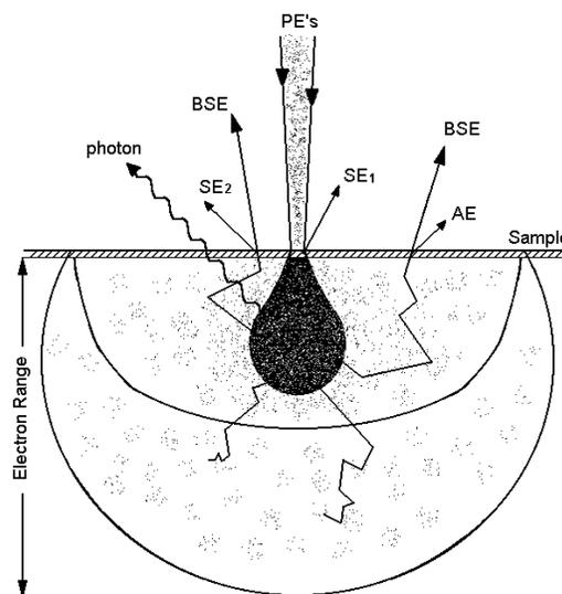
Figure 1. Physical processes resulting from energetic electron bombardment of a surface. Backscattered electrons (BSE), secondary electrons ( $SE_1$ ) produced by primary electrons (PE), secondary electrons ( $SE_2$ ) produced by BSE, Auger electrons (AE), and photons produced through inverse photoemission are shown. The hatched area shows the depth of predominant SE production [Reimer, 1993]. The shading shows the magnitude of the electron density.
