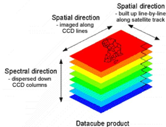
**Fig. 2. Hyper Spectral Imaging data**
