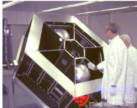
Figure 4 – AMSAT Phase 3D Satellite
