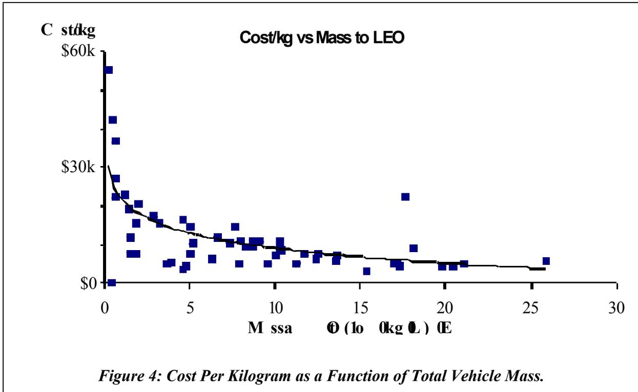
**Figure 4: Cost Per Kilogram as a Function of Total Vehicle Mass.**
