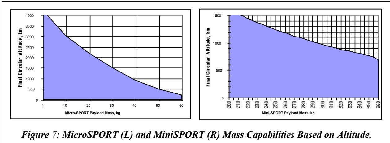
However, the Ariane 5 also has custom sized launch slots which can take large payloads, up to 1000 kg and more depending on the primary payload. The mass capacity of the MiniSPORT is shown on the right in Figure 7.
