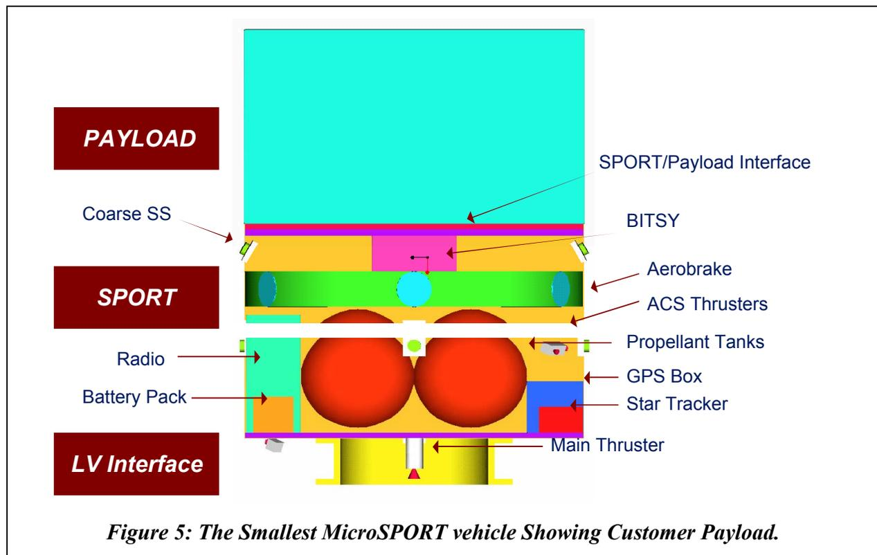
**Figure 5: The Smallest MicroSPORT vehicle Showing Customer Payload.**
