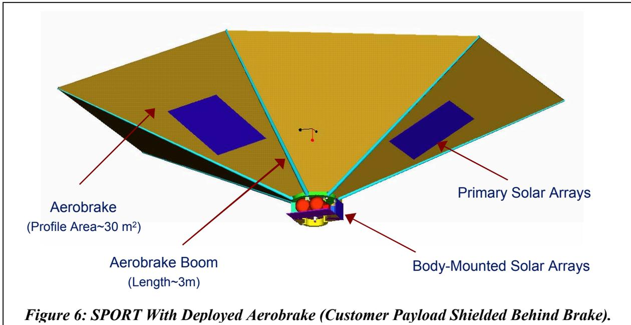
**Figure 6: SPORT With Deployed Aerobrake (Customer Payload Shielded Behind Brake).**
