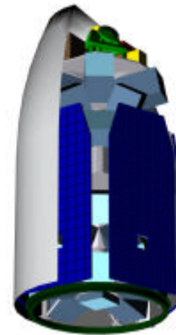
Figure 2. Stowed AXM Spacecraft Fits within Pegasus-XL Static Envelope
