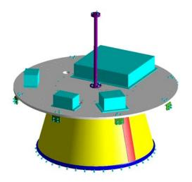
Figure 9 Starshine 3 Internal Structure
