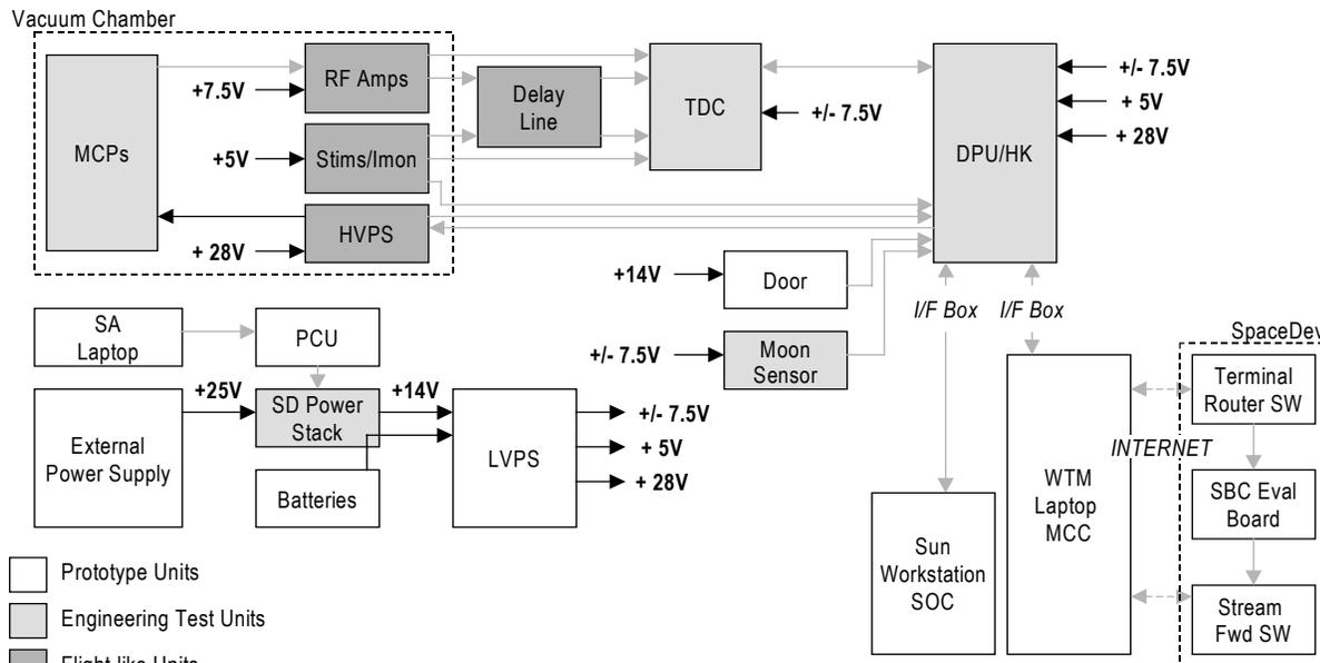
Figure 4: End-to-End Test Set-up and Interfaces
