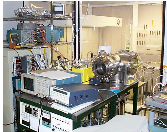
Figure 3: Detector Vacuum Chamber at UCB Facility
