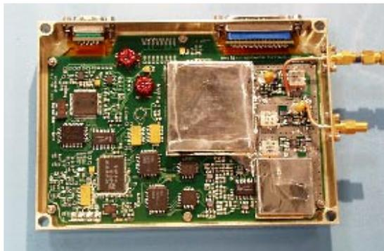
Fig. 5: SNAP-1 S-Band Downlink Transmitter
