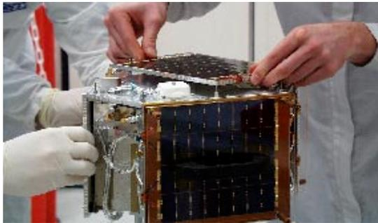
Fig. 2: SNAP-1 Solar Panels (4 in Total)
