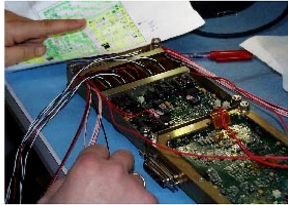
Fig. 3: The SNAP-1 Power System (Battery, BCR/PCM/PDM)
