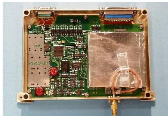
Fig. 4: SNAP-1 VHF Uplink Receiver
