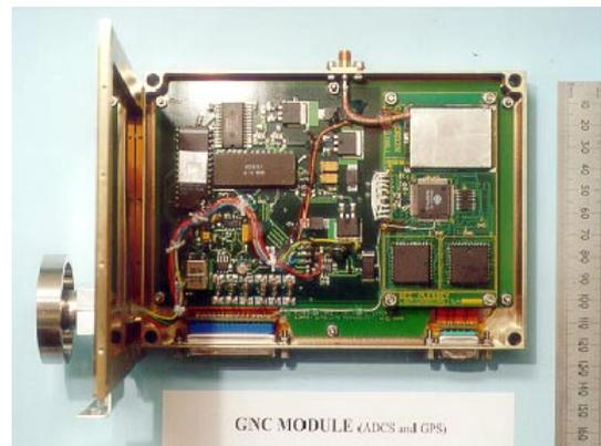
Fig. 6: SNAP-1 Guidance, Navigation and Control Module
