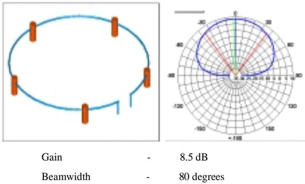
Figure 17: A Loop Antenna for the GPS/Telemetry Beacon
