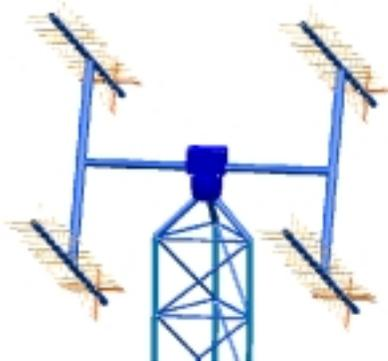
Figure 7: The Ground Station Uplink Antenna Array
