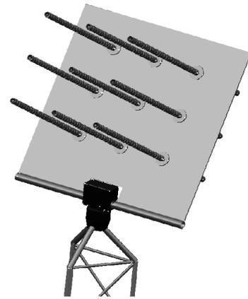
Figure 8: The Ground Station Downlink Antenna Array
