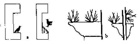
Figure 2. Wooden, metal or plexiglass covering over a ledge at a 45 ° (a) or porcupine wires (b) can be used to prevent roosting and nesting.
