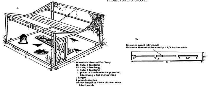
Figure 4. Starling decoy trap: (a) assembled view and (b) details of the entrance panel. Side and end panels are covered with wire on the outside; top panels are covered on the inside of the frame.
