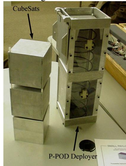
**Figure 8 - P-POD Deployer with CubeSats <sup>4</sup>**
