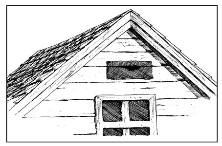
Figure 2. Bird netting is placed over the hole, and stapled tight along the top edge and down both sides. The bottom is left open. When the bats leave they hit the netting and crawl down the siding and out the open bottom. When they return they are unable to fly back up under the netting, and cannot return to their roost.
