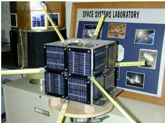
Photo 2. Personal Communications Satellite (PCsat) with Antennas
