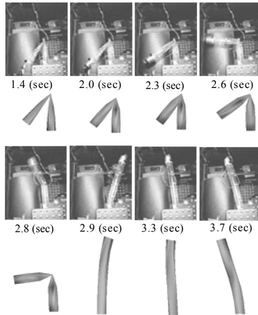
Figure 7. Deployment of a tube under micro-gravity
