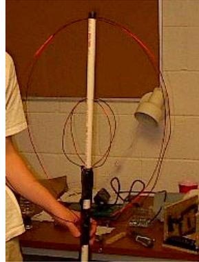
allowed the antenna to hang down from the payload, around the Solo Spirit fuel tanks and below the capsule, thus allowing a full 360° communications range. The software was designed to encode the data/images in UUencoding and transmit it to ground stations who would use ProComm (a shareware software program) to download the text. The ground stations would then log the text in a file and e-mail it back to control in St. Louis where the UUencoding would be decoded.
