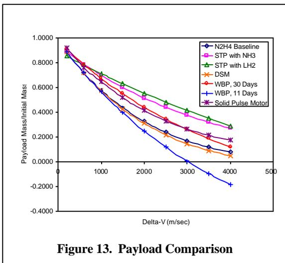
**Figure 13. Payload Comparison**
