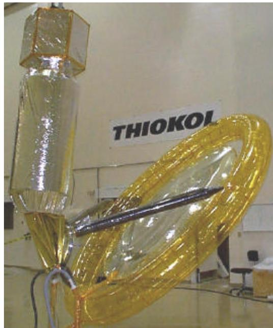
**Figure 2. Subscale STP Deployment Test**
