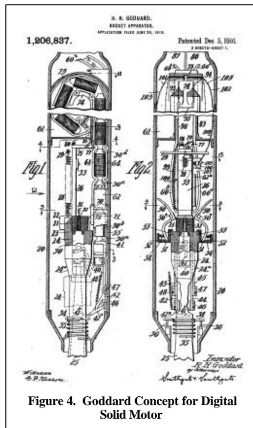
Figure 4. Goddard Concept for Digital Solid Motor
