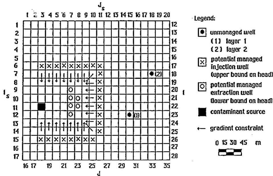
Figure 6 Head-difference constraint locations applied within the S/O model in Scenario 1.
