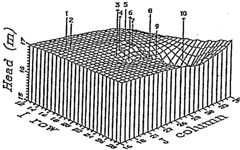
Figure 10 Subsystem potentiometric surface resulting after 6 months of optimal pumping for Scenario 1 (meters above MSL).
