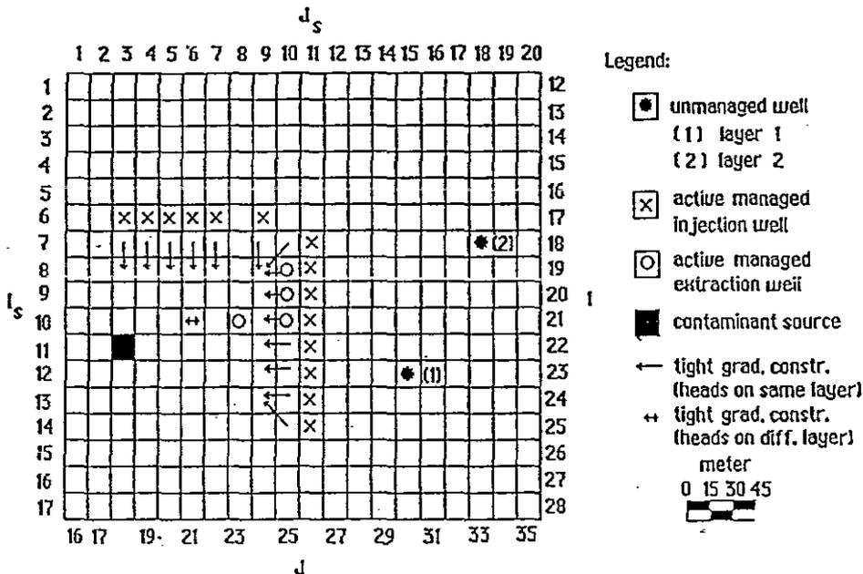
**Figure 11** Location of optimal pumping wells and tight head-difference (gradient) constraints for Scenario 3.
