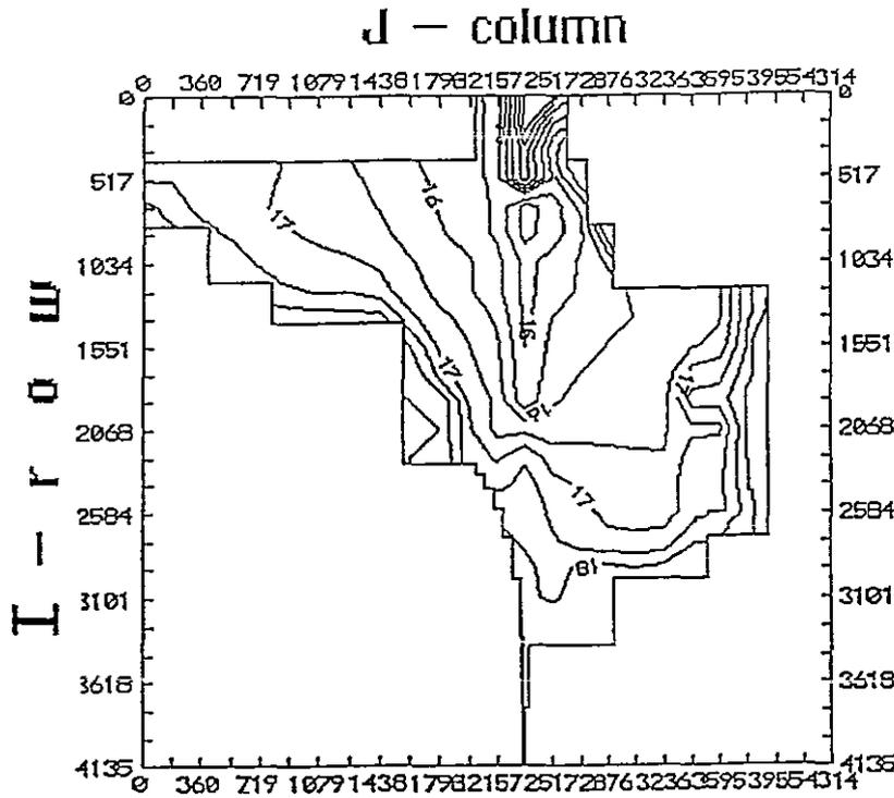
Figure 4 Nonoptimal (unmanaged) steady-state potentiometric surface contour map for the study area of Scenario 1 (meters above MSL).
