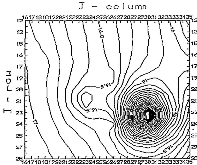
**Figure 9** Subsystem potentiometric surface resulting from implementing the optimal pumping strategy for Scenario 1 (meters above MSL).
