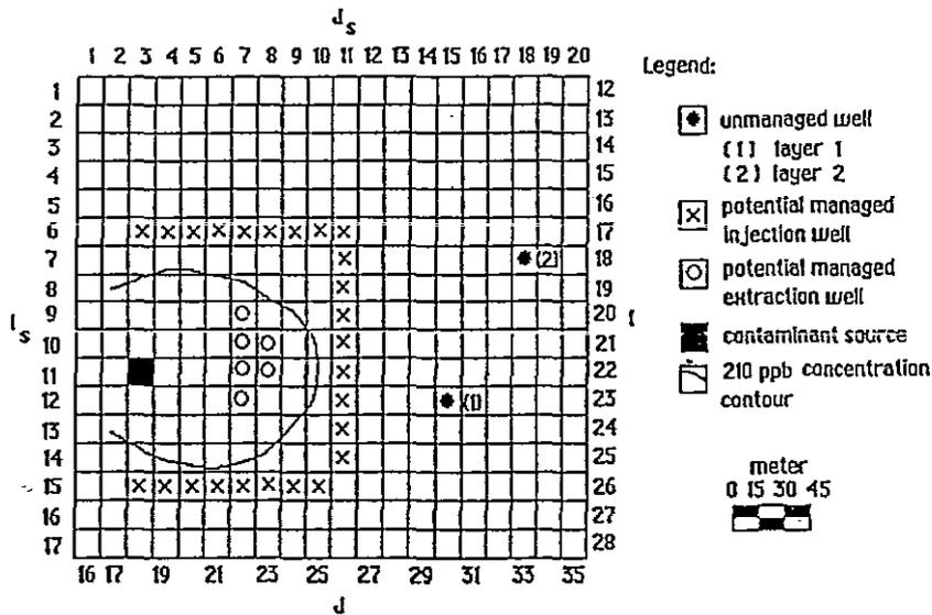
Figure 5 Subsystem discretization, potential well locations for Scenario 1, and 210 ppm contour, 60 days after contamination begins.
