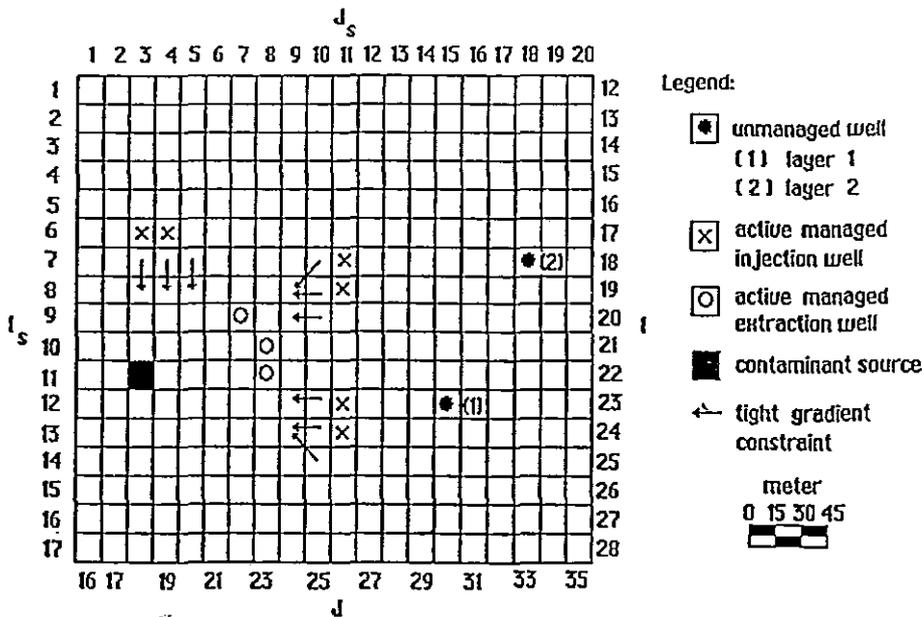
**Figure 7** Location of optimal pumping wells and tight head-difference (gradient) constraints for Scenario 1.
