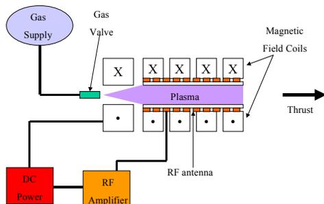
Figure 1. The RF Plasma Thruster
