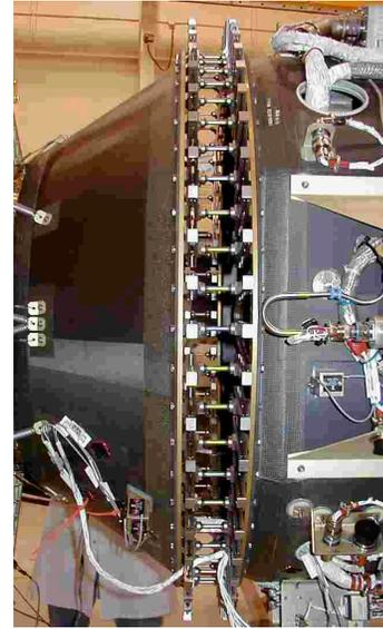
Figure 5 Typical installation of SoftRide MultiFlex
