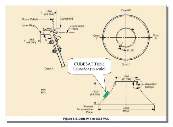
Figure 8 - CubeSat on Delta IV<sup>8</sup>
