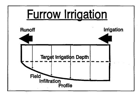
FIGURE 1. Infiltrating Water Depth in Furrow Irrigation
