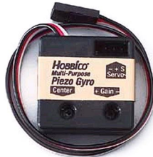
Figure 4.5: Hobbico Super Small Multi-Purpose Micro Piezoelectric Gyroscope
