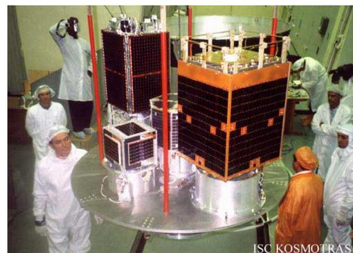
**Figure 5.** Platform with 5 spacecraft (Dnepr launch # 2)
