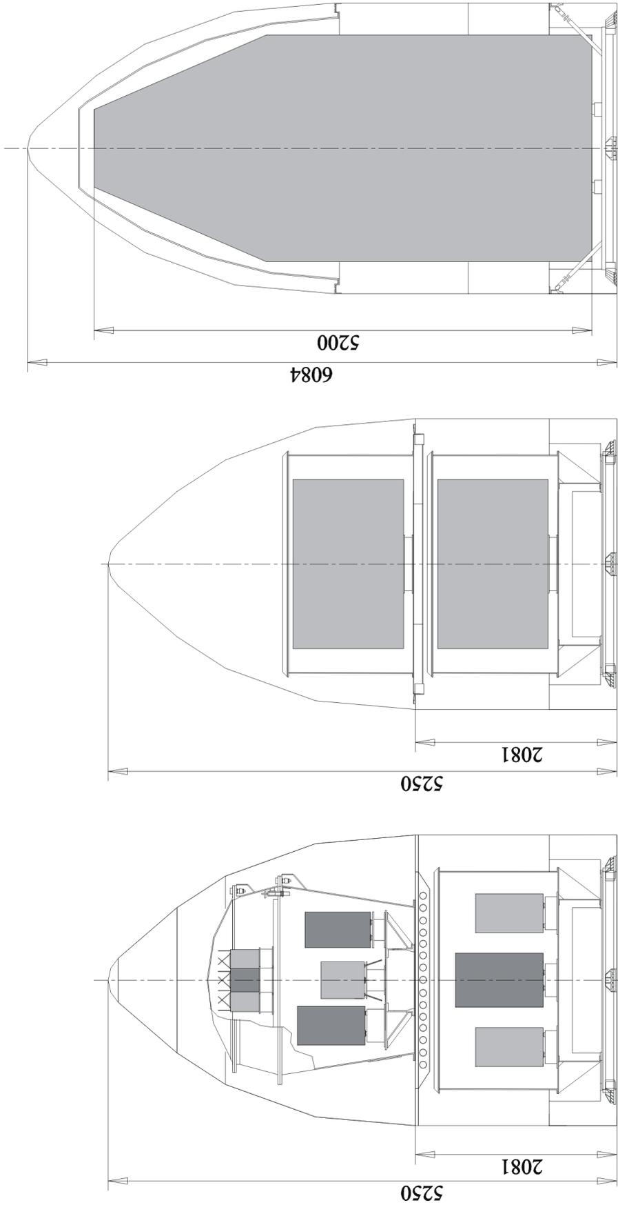
Fig.4 Variants of Payload Layout Within Dnepr-1 Payload Envelope
