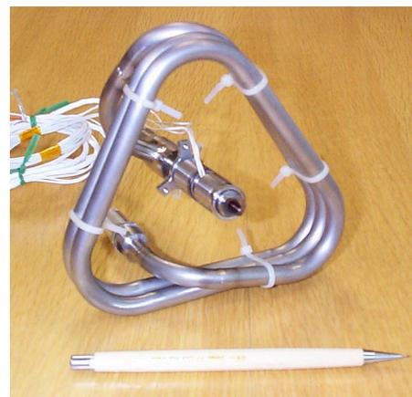
**Figure 3: SNAP-1 Pipework Assembly**
