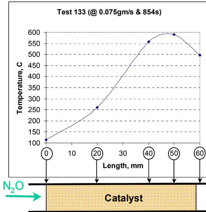
Figure 5: Axial temperature distribution. (Data are taken at 14<sup>th</sup> min. of the test. Mass flow rate is 0.075gm/s)
