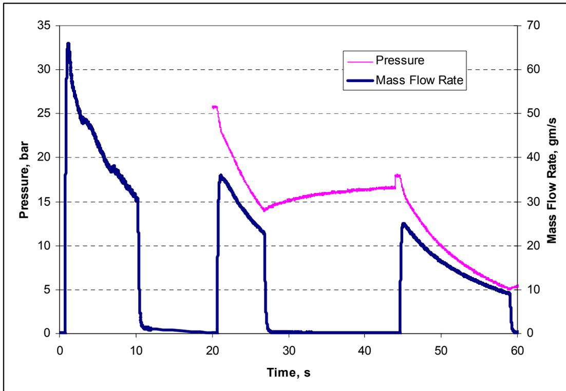
Figure 14: Nitrous oxide blow-down test.
