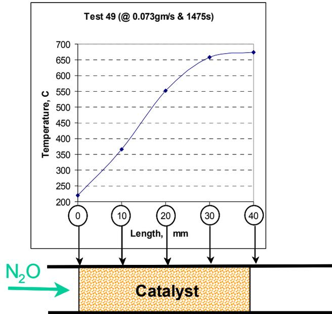
Figure 4: Axial temperature distribution. (Data are taken at 25<sup>th</sup> min. of the test. Mass flow rate is 0.073gm/s)
