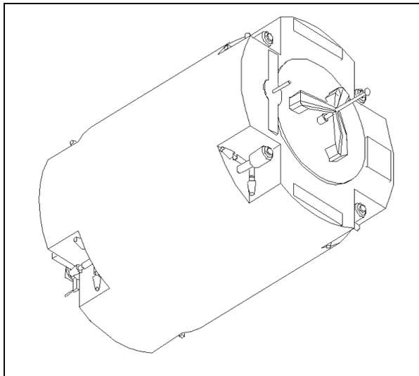
**Figure 4. Orbit Transfer Vehicle Conceptual Design, Rear View**
