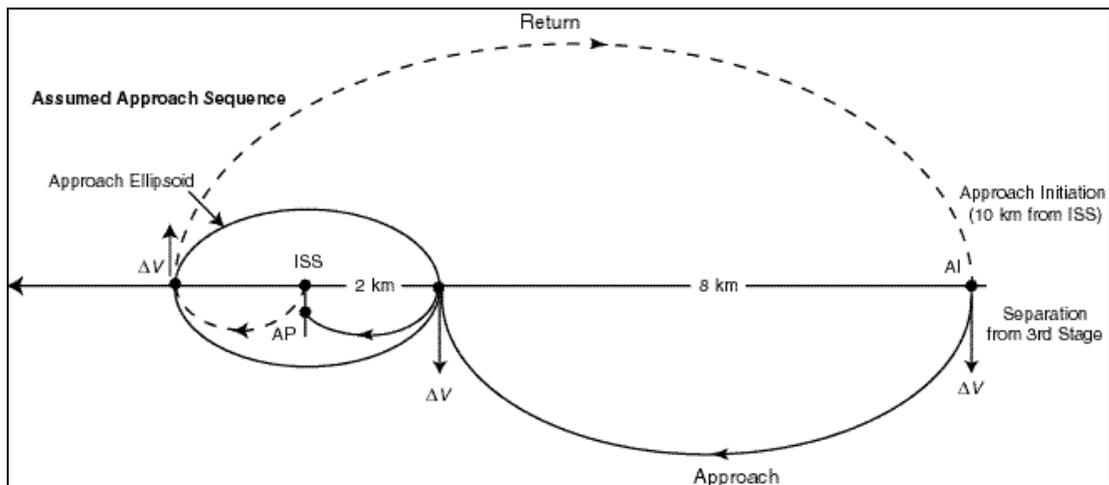
Figure 1. OTV Approach to ISS and Return Sequence
