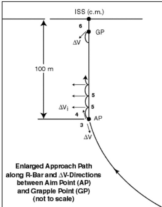
**Figure 2. Details of R-Bar Final Approach Path**
