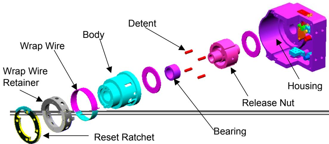
Figure 8. Exploded view of Release Mechanism. Major functional components are identified.
