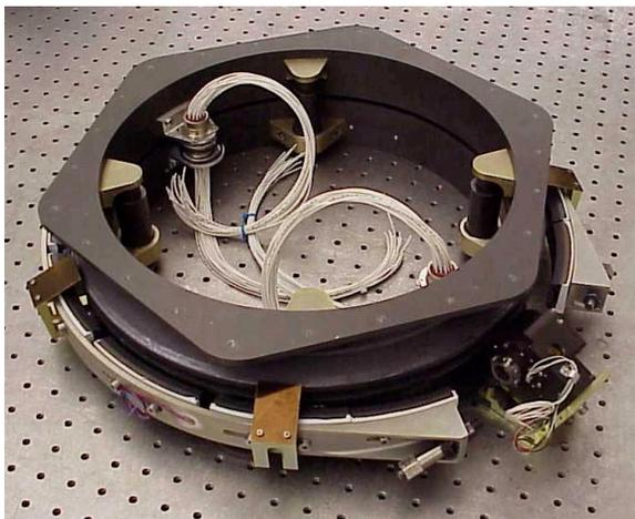
**Figure 2.** Nanosat configuration of clamp band system.
