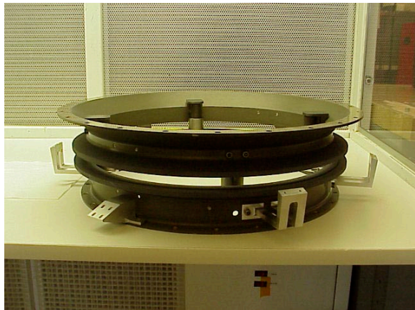
Figure 4. Primary structural components for the ESPA application.
