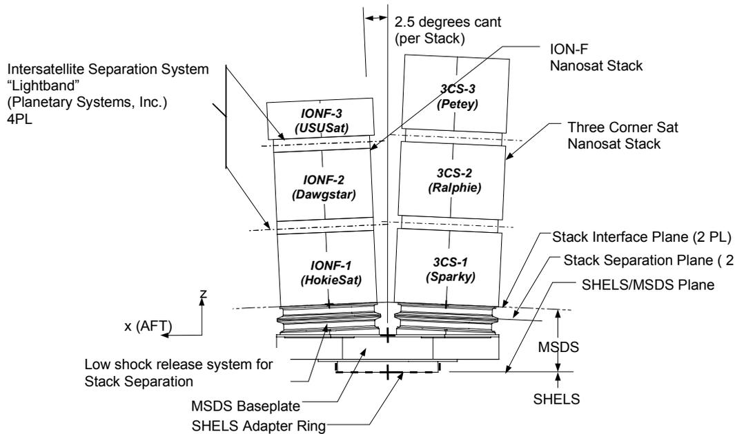
**Figure 1.** Nanosat launch configuration. This approach utilizes two stacks of small spacecraft on a single releasable platform.
