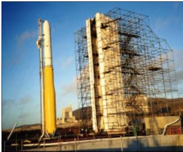
**Figure 16 - Minotaur with Thermal Blanket and Retracted Scaffold**
