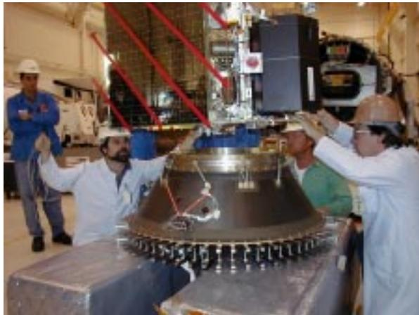
**Figure 12 - JAWSAT-to-PAF Integration**
