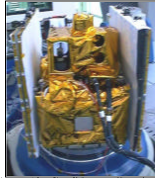
Figure 19. Confidence vibration testing
