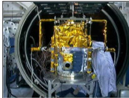
**Figure 18. Thermal vacuum testing**
