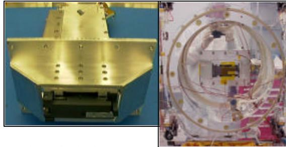
Figure 8. PicoSats launch from base of MightySat II.
