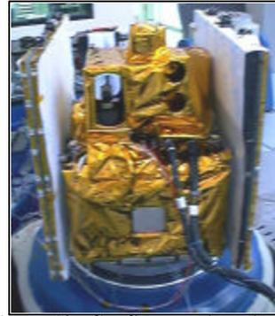
Figure 19. Confidence vibration testing
