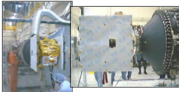
Figure 20. MightySat II attached to 4<sup>th</sup> stage of Minotaur 2.
