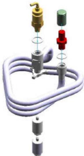
Figure 6 : Exploded view of propulsion assembly
