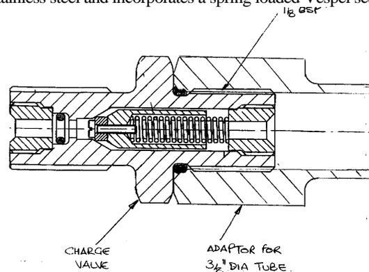
Figure 5 : Section view of the Fill Valve
