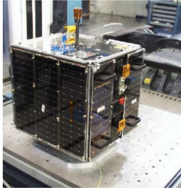
**Figure 2: STRV-1c under vibration test**
