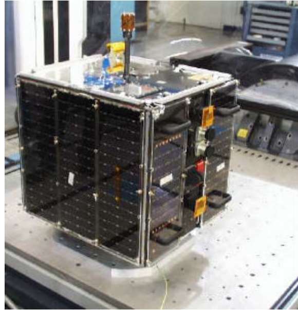
Figure 2: STRV-1c under vibration test
