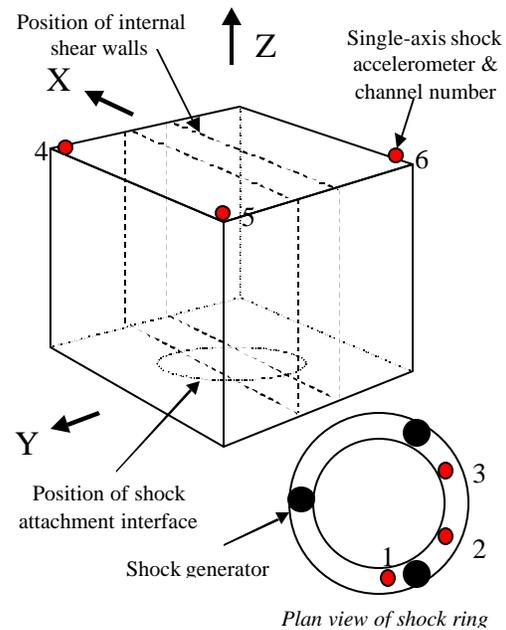
Figure 9 Shock accelerometer locations
