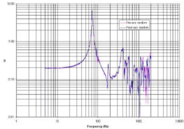
**Figure 12 Low-level sine response (pre- & post-X)**
