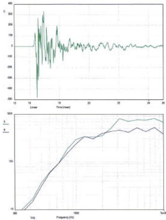
**Figure 14 Response to input shock and SRS**
