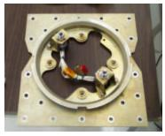
Fig. 10: The ØRSTED separation system
