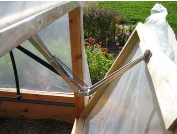
Figure 7. Vent opener doing its job on a sunny day.
