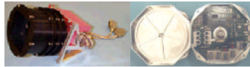
Figure 15 Surrey Flight Proven ADCS Hardware: Star Camera (left), Reaction Wheel (right)
