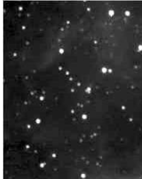
Figure 6. Image obtained from a Matsutov-Bowers Star Tracker with a 7 degree field of view.
