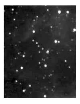
**Figure 6.** Image obtained form a Matsutov-Bowers Star Tracker with a 7 degree field of view.
