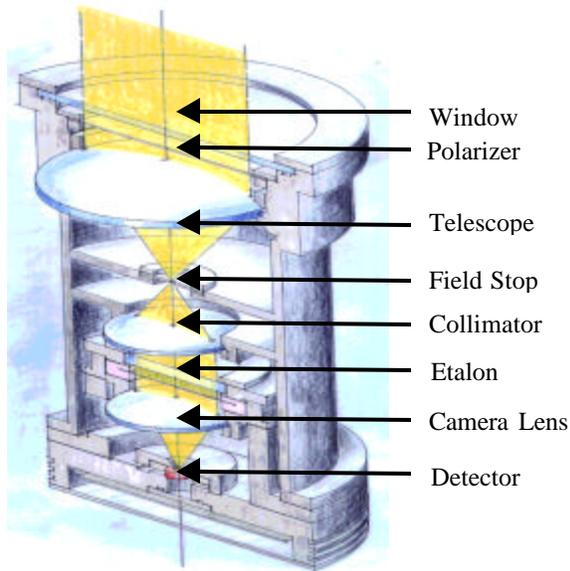
Figure 5. Cut-away view of the Prototype II.
