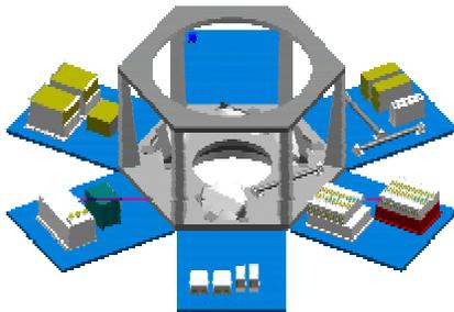
On the upper face, the Payload Interface Panel (PIP) carries the payload. For pointing performances, the PIP is made of CFRP, quasi iso-statically mounted on the bus; furthermore, attitude sensors are accommodated directly on the PIP.
