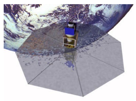
Figure 1. SPORT Configuration with Deployed Aerobrake
