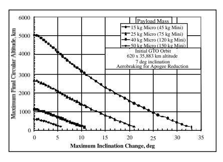
Figure 3. SPORT Aerobraking Performance
