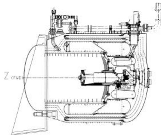
**Figure 3: WIRE Instrument Showing Telescope and Two-Stage Cryostat**
