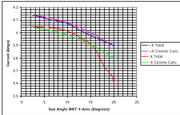
**Figure 11: Plot of solar array current vs. sun angle at 31 V, on day 159.<sup>10</sup>**
