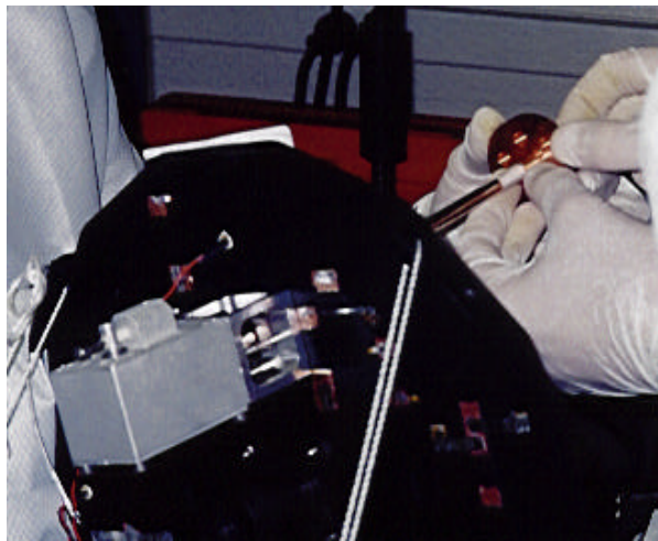
Figure 5. Final winding of boom element
