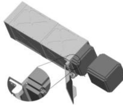
Figure 4.4.1: P-POD releasing CubeSats with rail detail.
