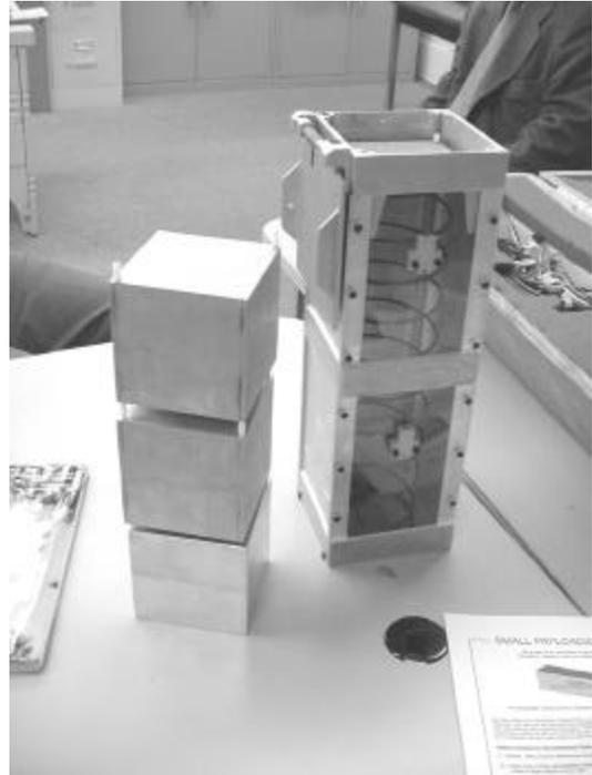
Figure 3.1 Prototype CubeSat Launcher and Mass CubeSat Models
