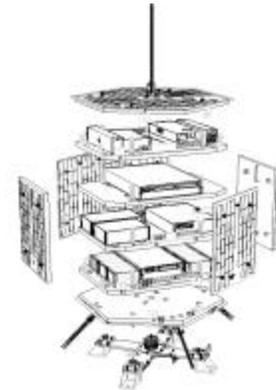
Figure 2.2 Stacked Module Concept
