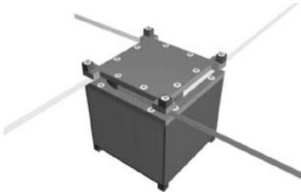
Figure 4.4.4. The PolySat with Deployed Dipole Antennas
