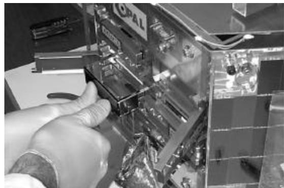
Figure 2.6 Loading a Picosat into OPAL
