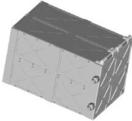
Figure 4.4.2 Four P-POD's in a 2x2 configuration
