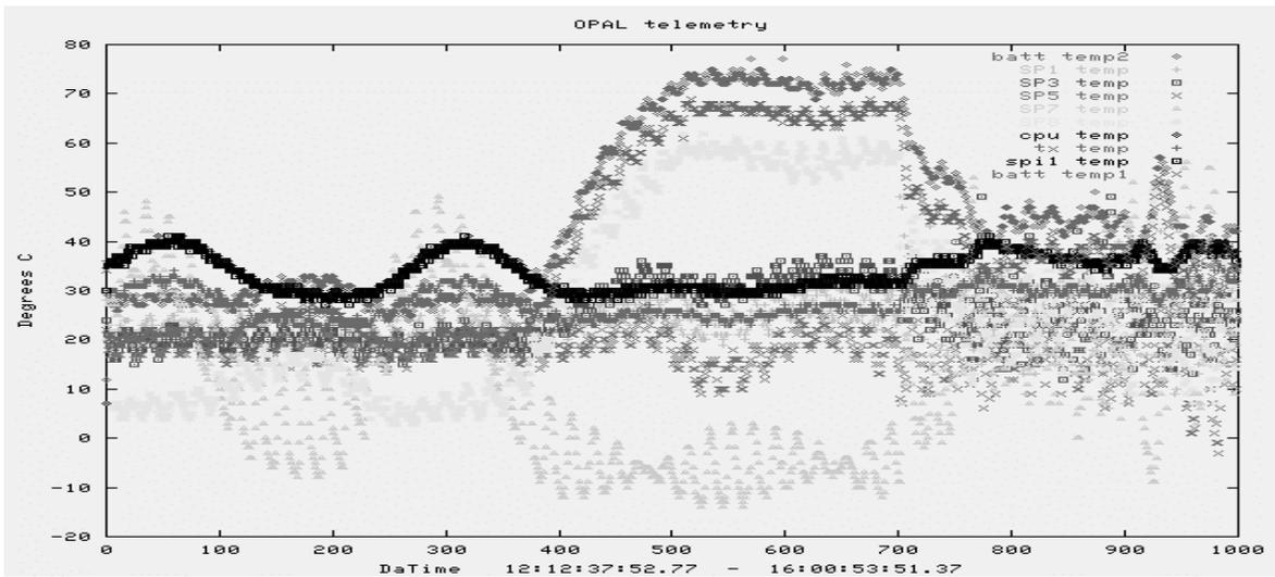
Figure 2.8 OPAL temperatures before and after picosat launch
