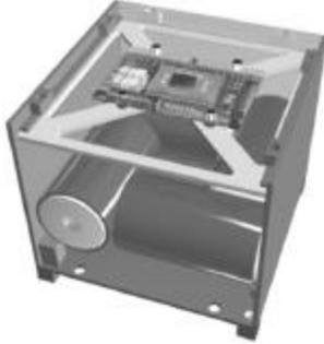
Figure 4.4.5 Disassembled CubeSat Showing Batteries and Electronics Tray
