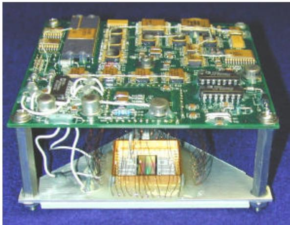
**Figure 1. Top View of the CCD Experiment Board**
