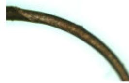
Figure 14. Etched BeCu Wire
