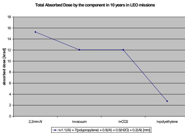
Fig.16- Total Absorbed Dose for a NEGESAR-based Equipment in LEO missions
