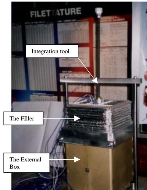
Fig.6- The SMALL DEMONSTRATOR in the integration phase
